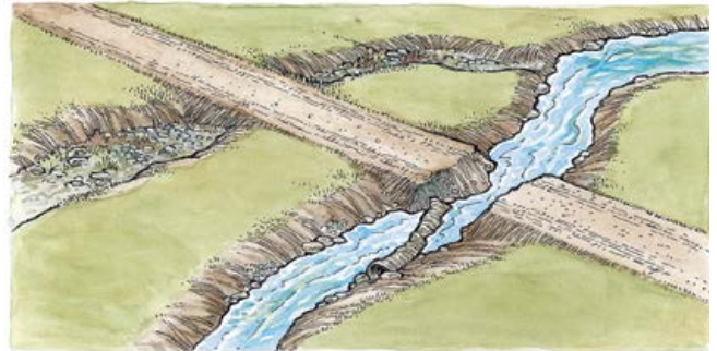
Early road construction techniques often filled side channels, contributing to the failure of main channel culverts during high water.
