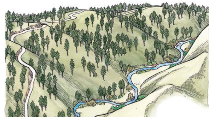
BEST OPTION. Build road on ridge top and plan for cable harvesting.
