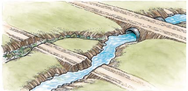
In this example, a minor relocation of the road prism resulted in only one culvert reinstalled for road access. This reduces maintenance and allows the side channel below the new crossing to be restored to a more natural condition.
