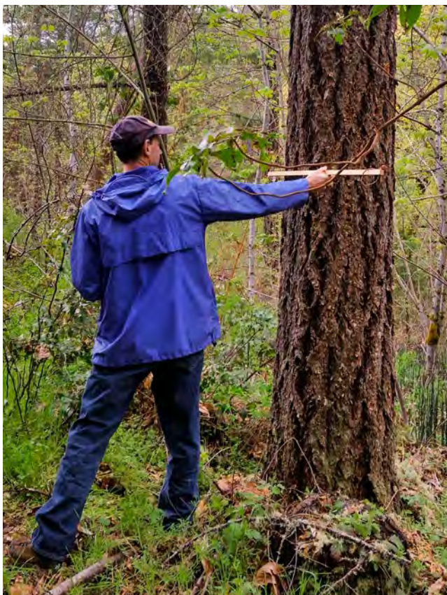
A landowner measuring the DBH of a tree using a Woodland Stick.
