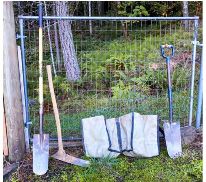
Specialized tree-planting tools, from left: long-handled planting spade, hoedad, tree planting bag, short-handled planting spade.
