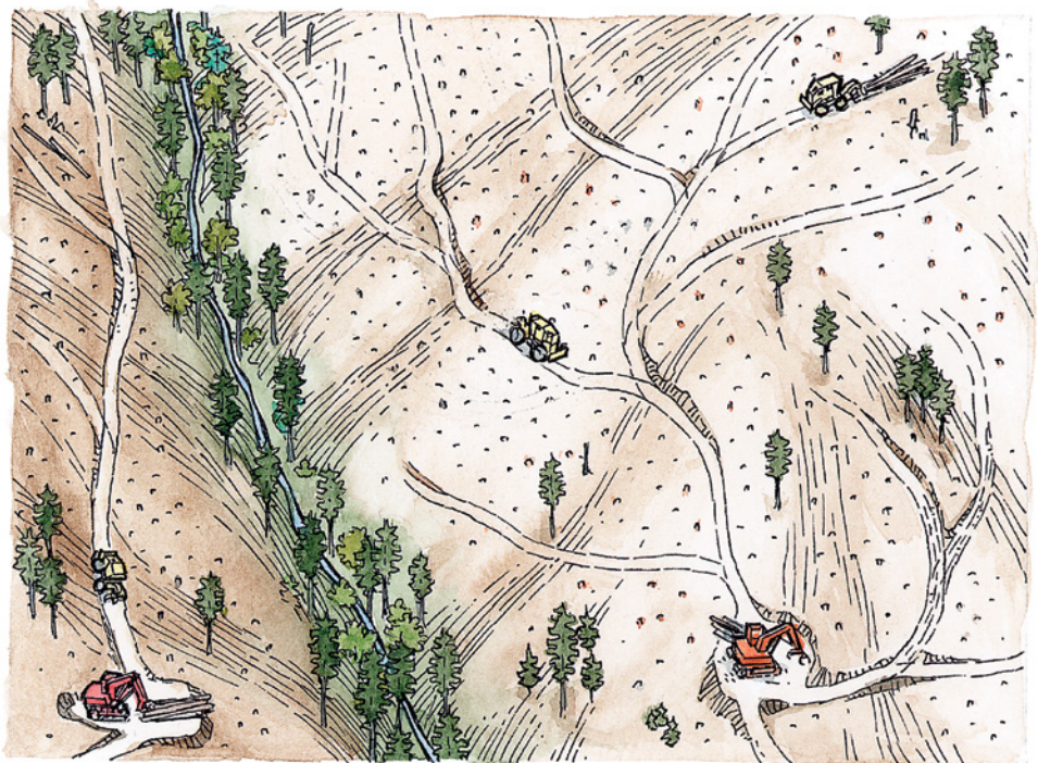
On steeper slopes, the parallel skid trail pattern attempts to parallel the land's natural contours.
