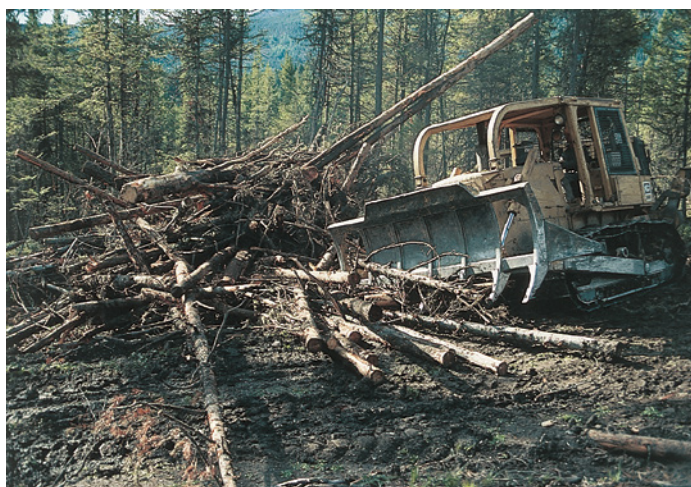
Slash piles free of soil burn cleaner, reduce soil erosion and protect productive topsoil.
