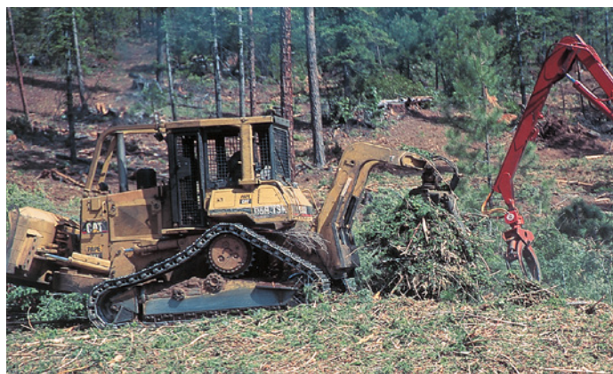
The same machine that brings whole trees to the landing may carry slash back and scatter it on the forest floor. This returns nutrients and organic matter to the soil for the next forest. It also protects soil from erosion, especially in skid trails. The fire hazard is minimal because the slash is crushed and close to the ground.
