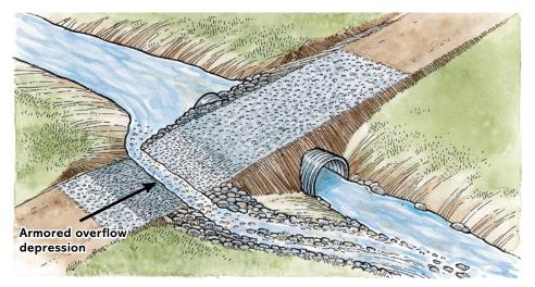
This vented ford is a cross between a ford and a culvert crossing. Water passes through the culvert during normal flows, but the structure can accommodate peak stream flows across a ford section during large storms. Any permanent culvert in a stream needs to be sized for the 100-year peak flow.
