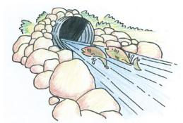
Fish may not be able to swim fast enough to overcome culvert water velocity that develops in culverts narrower than the width of the stream. Rule of thumb: Water moving through a bare culvert that is turbulent (uneven water surface or whitewater) is probably a fish-passage barrier.
