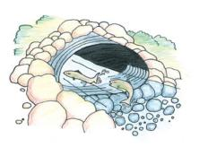
Water may be too shallow for fish to swim. Bare pipes frequently result in shallow water, leaving fish only partially submerged and unable to get maximum thrust from tail and body movements.
