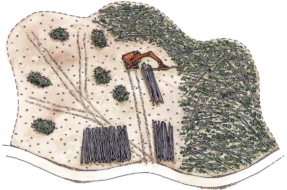
Shovel logging starts at the nearest access point and moves logs until they are within reach of the road. From there, they can be loaded onto trucks.
