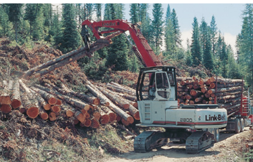
The loader serves two needs: loading trucks and piling tops, branches and log chunks for later burning, chipping or other uses.
