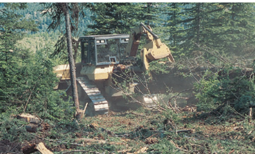
A crawler tractor or skidder with a grapple picks up the bunched trees and drags them to a landing or roadside. Some grapples can swing 180 degrees, making it easier to operate in tight spaces.
