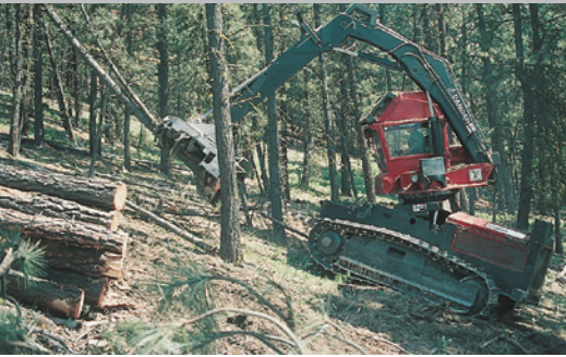
A feller-buncher severs trees and lays them in bunches with limbs and tops attached. These bunches are oriented with tree trunks facing downhill.
