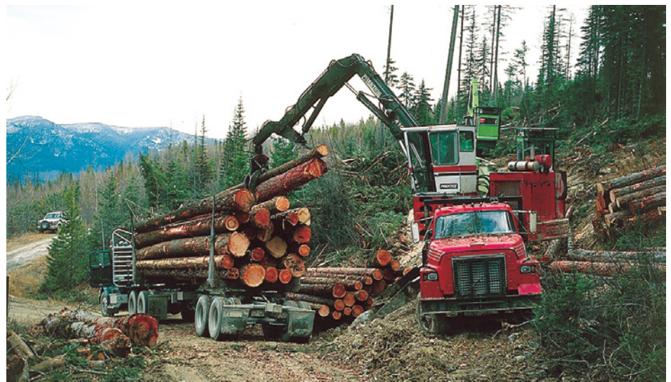
At the landing, a log loader moves logs onto trucks for delivery to the mill.
